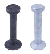
The Capstan Anchors are a safe, simple and effective system for lifting most types of precast concrete units. The anchors are hot drop forged from high grade steel and, provided the anchor is specified and installed correctly, ensures safe and secure lifting, turning and transportation of units.
