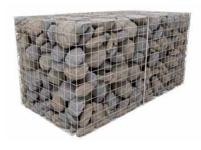
Gabions are wire mesh baskets manufactured from 3.0mm Galfan Wire, and are filled on site with typically stone or rock to form larger building modules. Galfan wires are best used where the additional PVC coating is not a requirement, such as freshwater river applications and low height retaining walls on dry land, where aesthetics are not paramount.
