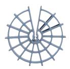
Minifix Wheel Spacers have clamping tongues to accommodate a variety of bar diameters. They have an open design which does not interrupt the concrete flow, and outside ribs which minimise contact with the formwork.
